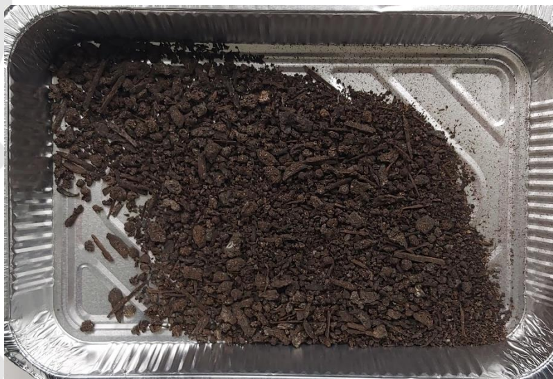
Figure 21. Sieved substrate of the sample with test material at the end of the disintegration test.
