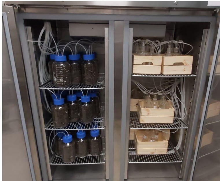
Figure 4. Picture of the vessels in the climatic chamber for the biodegradation test in composting condition.
