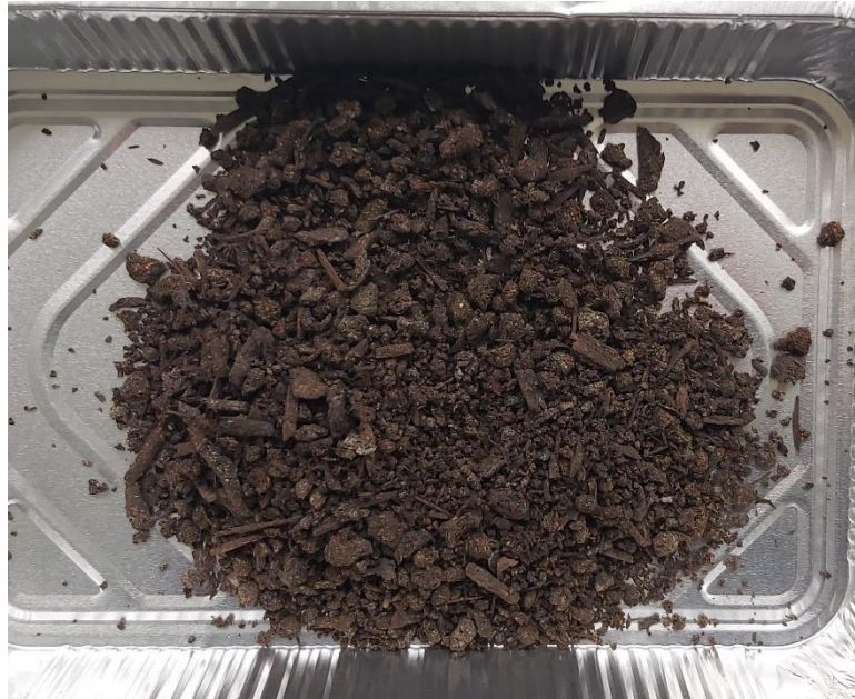
Figure 20. Sieved substrate of the sample with blank compost at the end of the disintegration test.
