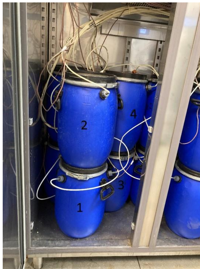
Figure 10. Pictures of the equipment for disintegration test.
