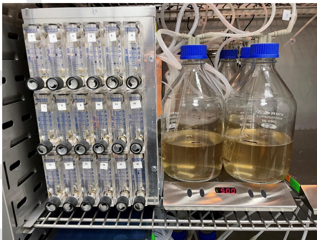
Figure 2. Picture of the biodegradability test set-up
